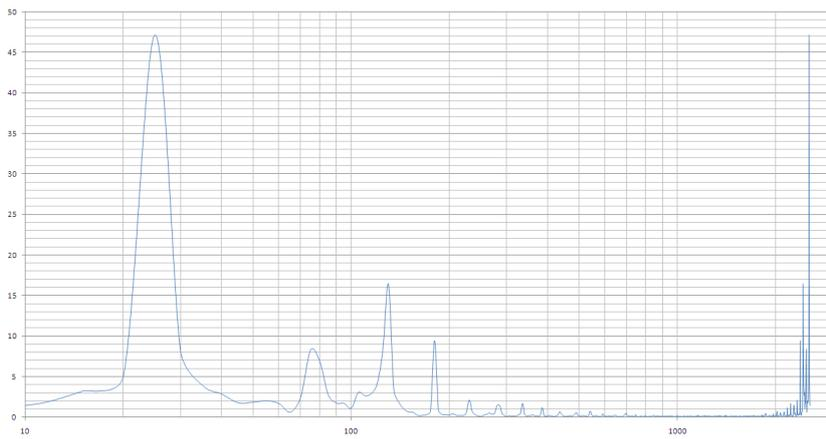
Figure 6: FFT of rectifier current waveform
