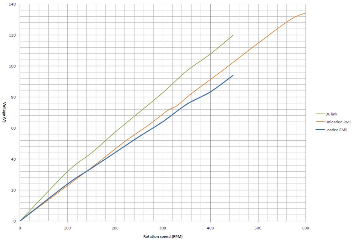
Figure 8: Voltage against RPM
