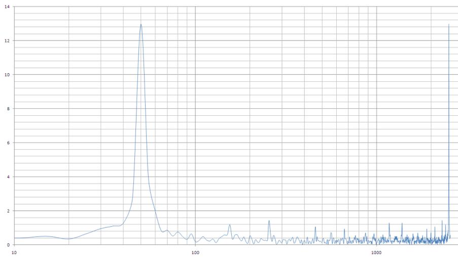
Figure 4: FFT of 230v output current waveform
