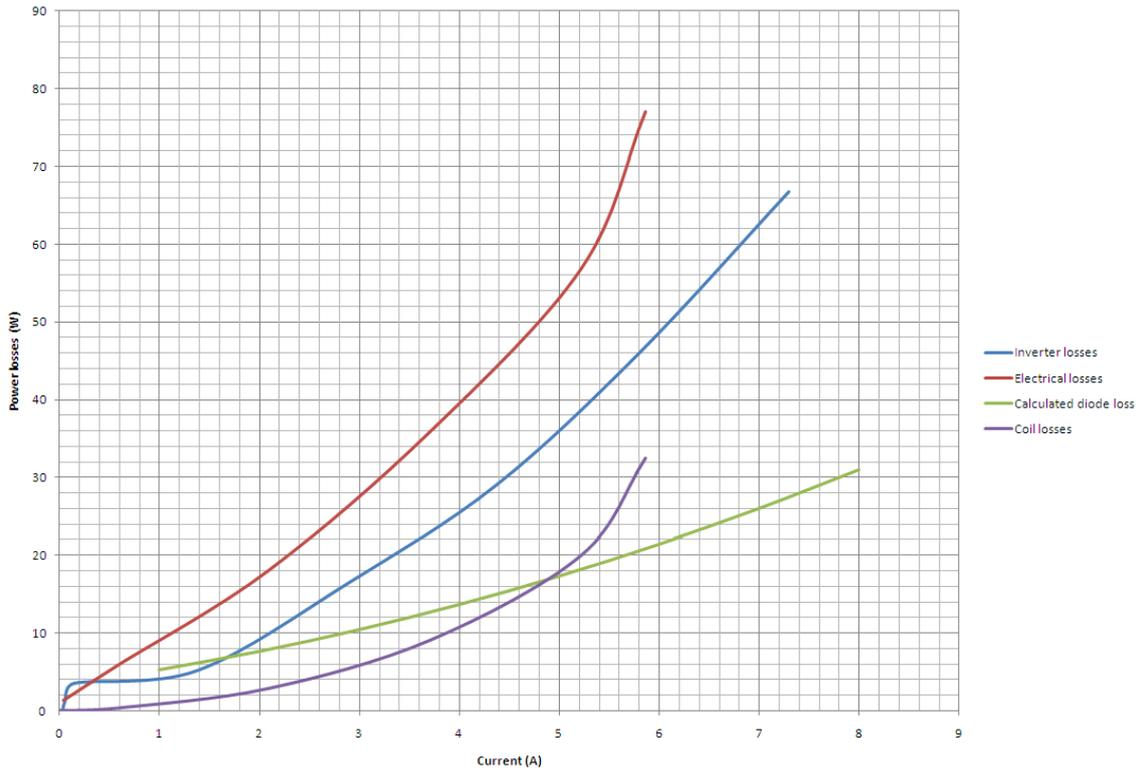
Figure 13: Power loss against current
