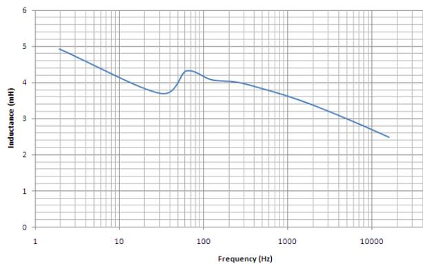
Figure 1: Stator inductance (line - line)
