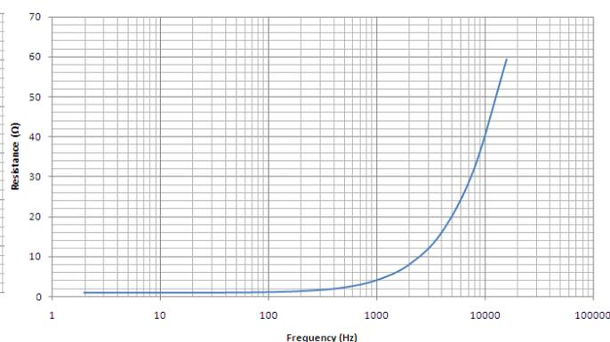
Figure 2: Stator resistance (line - line)
