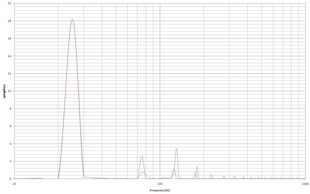
Figure 9: Theoretical coil losses (blue) and square wave losses (red) due to current harmonics
