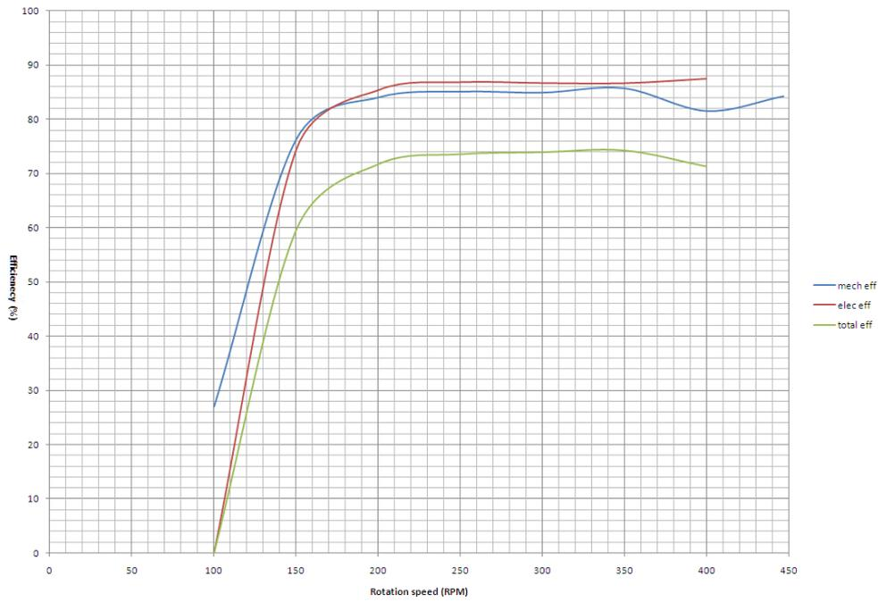
Figure 10: Speed against efficiency
